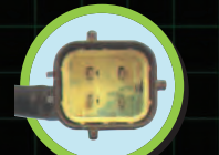
Replace with new sensor. Check connections and seal.
