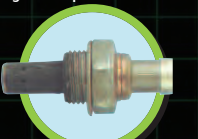
Diagnose and correct fault. Note: Excessive deposits of soot and oil on the protective sleeve are not caused by the sensor itself.
